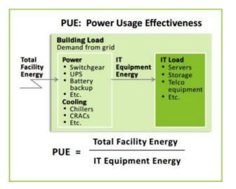
This PUE will also need to be verified in relation with section 1-3 on Energy Efficiency and Performance Verification. For verification purposes, if UPS output data is not available, the closest direct measured power data will be used and a fixed PDU loss will be applied based on industry norms for such equipment.
