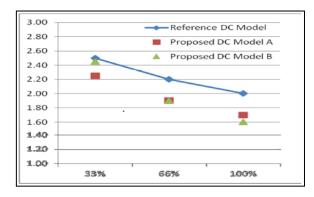
**DC Model A:** Full Load PUE =  $1.7 \rightarrow 16$  pts At 66% Load, % Improvement = 13.64 > 75% of 15; At 33% Load, % Improvement = 10.0 > 50% of 15; **Credits** = 1.0x16 = 16
